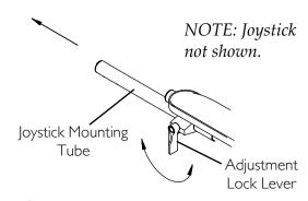
**FIGURE 5.8** Preparing the Joystick for Use
